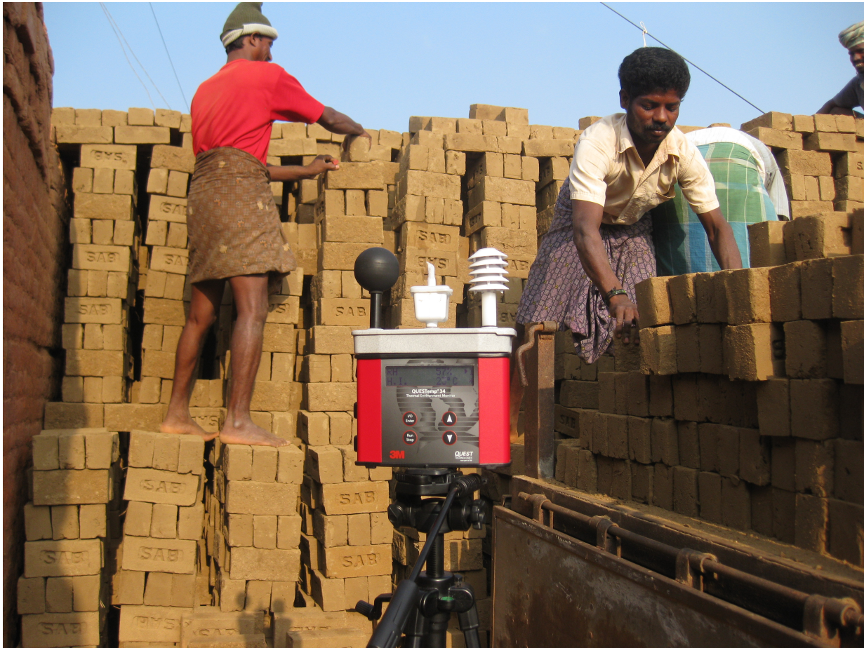
Figure 1. Picture of a WBGT measurement instrument (QUESTemp) at one of the brick kilns studied [K. Lundgren Kownacki, 2018].
